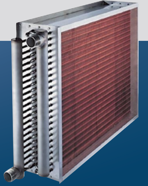
Water Coil used in BWR drywell. Stainless steel tubes, stainless steel removable header, and copper fins.
