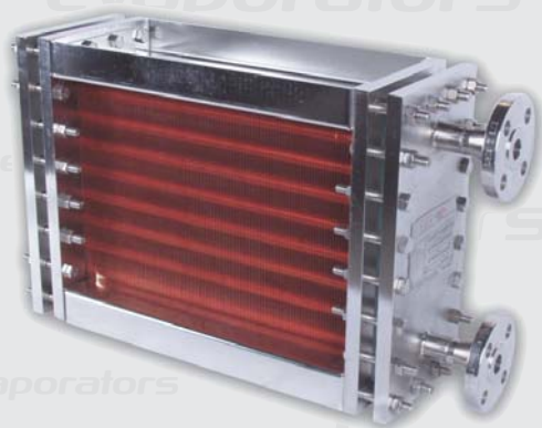
Stainless steel, ASME Section VIII, Division 1 "U" stamped, electro-polished chilled water coil with copper fins and removable cover headers. This design is used where optimum thermal efficiency must be maintained and minimal down time is critical.
