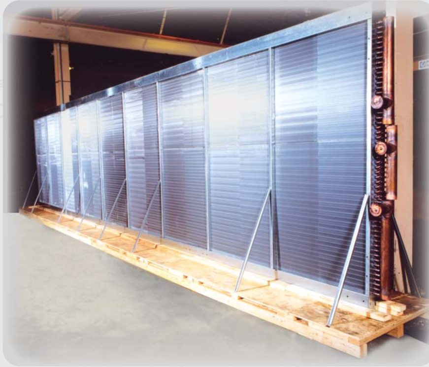
84"x 384", multi-stage condenser coil with copper tube and aluminum fin construction. This coil was exported to Hong Kong as a replacement for an existing rooftop installation.
