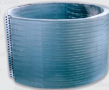
Large face area 3/8" OD copper tube and aluminum fin condenser coil for a condensing unit application. The circular shape occupies a small footprint, and the open center section houses the fan and compressor.
