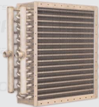
All stainless steel polypropylene glycol-cooling coil with stainless steel plate fins spaced at 1.5 fins per inch to handle severe frost buildup. This coil is used in refrigerated food processing.
