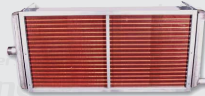
Three-row steam coil with stainless steel tubes, copper fins, and welded half-pipe header. This coil is designed for food processing smokehouses.
