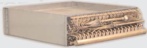
Copper tube evaporator coil designed for installation in a heat pump application for aircraft ground support equipment. The intricate refrigerant distribution tubing is held in close to the manifold to fit a confined space. Multiple headers and distributors permit coil operation in a variety of environments.
