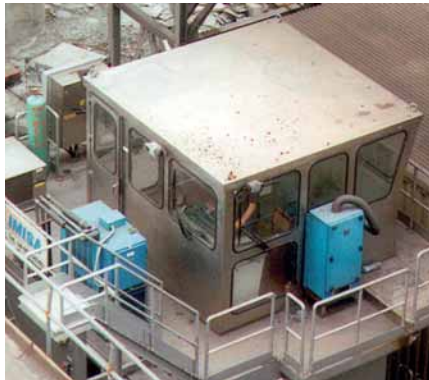
Lintern severe duty AC units on a crane control cab
